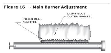
Main burner flame should form sharp blue inner mantel with no yellow.
