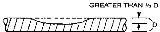
Figure: 5-2 – Repair Necessary. Significant Damage to the Tubing Due to Impact or Crushing
