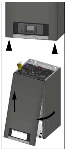
Figure 1 - Removing Housing
