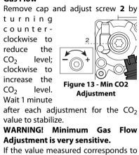
If the value measured corresponds to the value given in Table 3 adjustment is complete. Otherwise continue the setting procedure.
