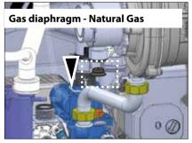
Figure 7 - Remove the NG-diaphragm
