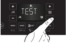
Wait 1 minute for the boiler to stabilize before carrying out the combustion analyses.
