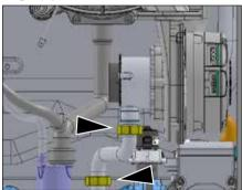
Figure 6 - Remove the gas pipe
