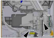
Figure 4 - Unhook the Junction Box support
