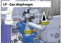
Figure 9 - Insert the LP-diaphragm
