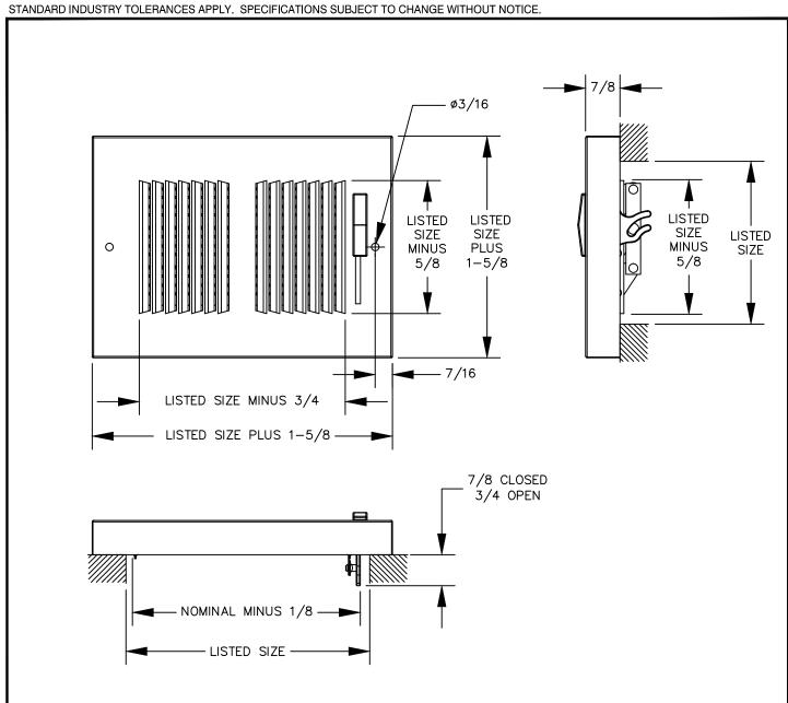
Model 667 is a stamped straight blade baseboard register with mounting holes. Constructed of steel with 1/3 inch fin spacing set at 45 degrees, it features a multi-louvered damper. Standard finish is white.
