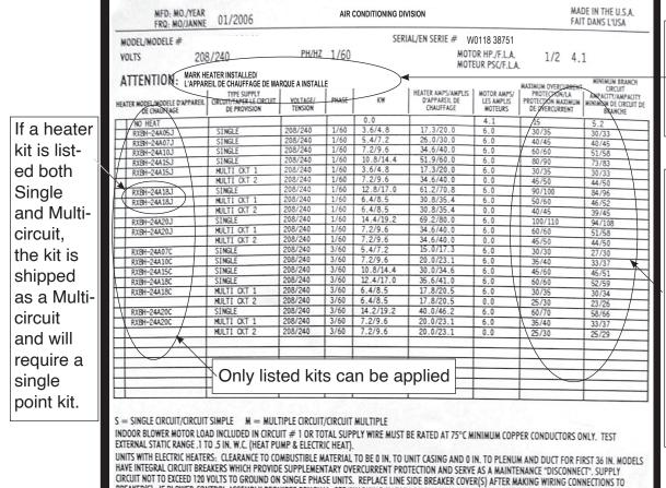
BREAKER(S). IF BLOWER-CONTROL ASSEMBLY REQUIRES REMOVAL, SEE "WARNING HAZARDOUS VOLTAGE"
