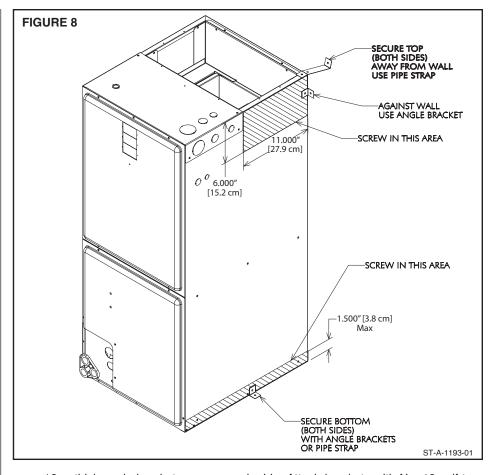
16ga thick angle brackets one on each side. Attach brackets with No. 10 self-tapping  $^1\!\!/\!\!2"$  [13mm] long screws to air handler and use  $^5\!\!/\!\!16"$  [8 mm] lag screws  $1^1\!\!/\!\!2"$  [38 mm] long to wall stud. Secure bottom of unit with two 16ga "L" brackets with No. 10 self-tapping  $^1\!\!/\!\!2"$  [13 mm] long screws to air handler and use  $^5\!\!/\!\!16"$  [8 mm] lag screws  $1^1\!\!/\!\!2"$  [38 mm] long to floor.
