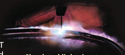
Simulated lightning test with no product failure
