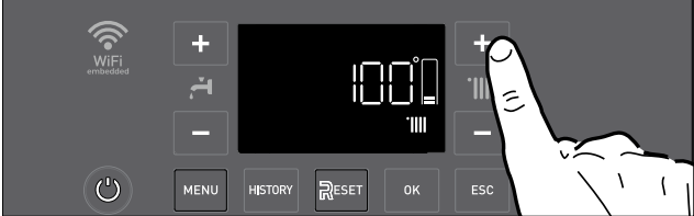
Figure 3 - Central Heating (CH) Temperature Adjustment
