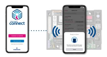
**Near Field Communication (NFC)** creates an interface between the control and your mobile device with the White-Rodgers Connect app. Place mobile device in contact with the NFC marking on module to enable a connection.
