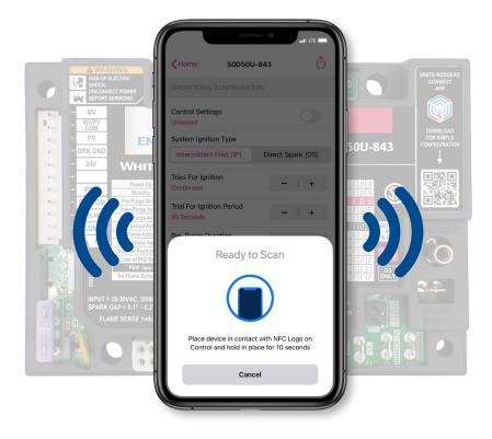
Place mobile device in contact with the NFC marking on the board to enable Near Field Communication (NFC) connection
