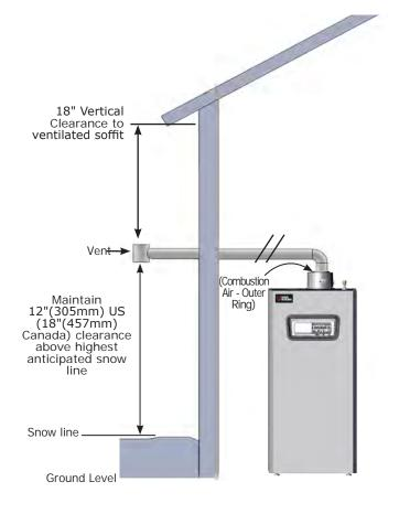
Combustion air and Vent Piping Length Page 22.
