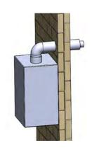
Twin Pipe – Figure Exhaust and intake air are separate pipes, can be terminated using single wall terminals from the vent manufacturer or field built configuration using elbows or tees.
