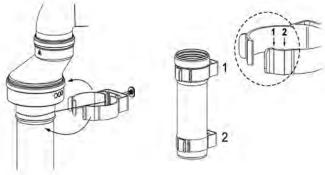
FIGURE 6-25 Maximum Distance Between Supports
