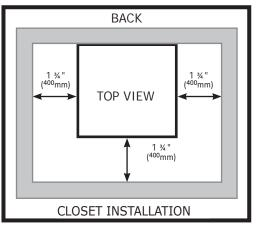
0 in. /0 mm between the Back of the Unit and the wall
