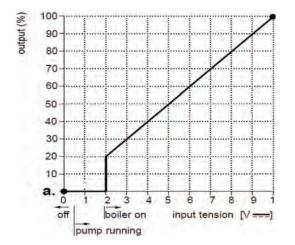
Dependent on minimum modulation depth (set speeds, standard 20%)
