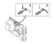
6. Analog Output - 0-10V - Temperature or heat output can be chosen for this feedback message. The two controls are described briefly below.
