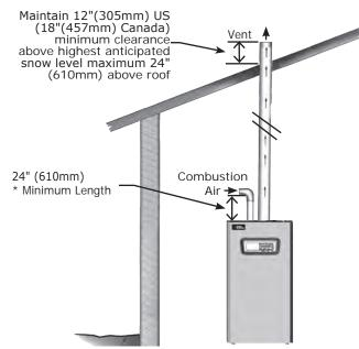
FIGURE 6-14 Flue on Sidewall, Inside Combustion Air
