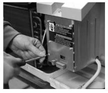
4. High voltage ballast should be mounted near or inside of the electrical controls.
