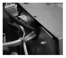
9. Check again to make sure that the all cordage is routed safely through the unit and does not interfere with unit operation, blower wheel, etc..
